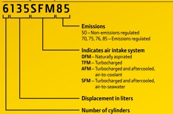
A John Deere marine engine model designated as 6135SFM85 is a 6-cylinder, 13.5-liter turbocharged and aftercooled, air-to-seawater engine that is emissions regulated.
